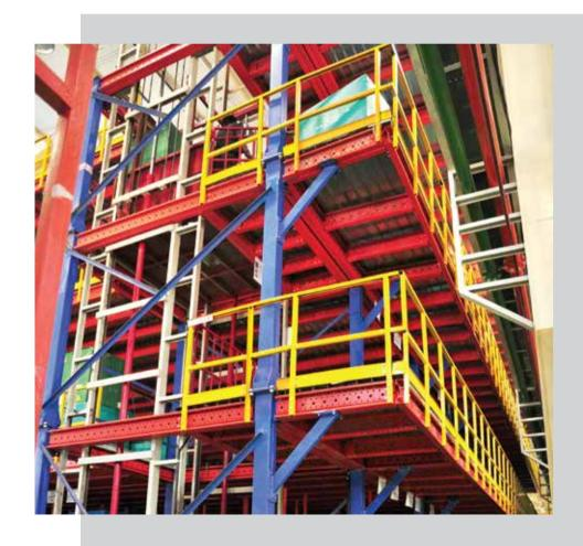
This type of storage systems adds more space to the warehouse to stack items high up. Mezzanine floors take maximum advantage of the height of premises, doubling or tripling the surface area. Mezzanine floors are totally dismountable & reusable & their structure, dimensions & location can be easily modified.
